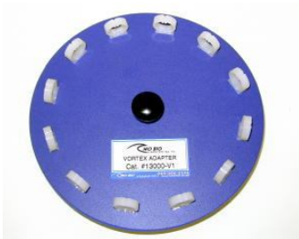
Vortex Adapter 13000-V1 Holds 12 (1.5 - 2.0 ml) Tubes
