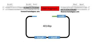
IG AmpR/KanR-pCR Vector is a linearized vector that has ampicillin, kanamycin-resistant genes and ccdB gene for removing self-ligated clones.
