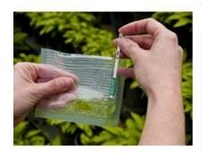
The *Acidovorax avenae* subsp. *citrulli* (*Aac*) ImmunoStrip® is used to detect the presence of *Aac*, the causal agent of bacterial fruit blotch, in watermelon, squash, pumpkins, and cantaloupe. The assay can be used to test leaves, fruit, bacterial cultures, and seedlings exhibiting symptoms of Aac. ImmunoStrips® are the perfect screening tool for use in the field, greenhouse, and the lab.
