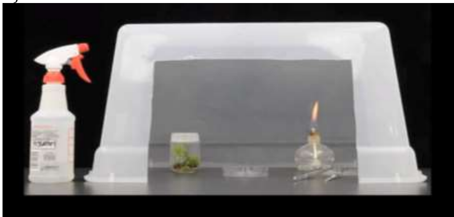
Figure 1. An example of a 'Still-Air Transfer Chamber'
